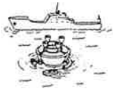
7 - SURFACE CRAFT SECURE AUXILIARY FLOATATION GEAR TO STAGE TO MAINTAIN ENGINE-UP VERTICAL POSITION.
