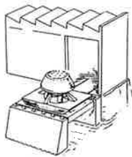
1 - ASSEMBLY & TRANSFER IS ACCOMPLISHED ON UNIVERSAL TRANSPORTER/ASSEMBLY FIXTURE. COMBINED UNIT IS MOVED ON ROLLERS ABOARD SYNCHROLIFT ELEVATOR FOR LOWERING TO DOCK BASIN WATER SURFACE.
