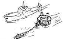
10 - N-I STAGE IN TWO. PURGE OF TANKS ACCOMPLISHED UNDERWAY. NECESSARY REPAIRS OF EMERGENCY NATURE MADE EN-ROUTE AS RESULT OF PRELIMINARY INSPECTION ACCOMPLISHED DURING STAGES 7-9.
