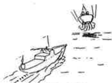
6 - PARACHUTES & RETRO ROCKETS USED TO SLOW RATE OF DESCENT. HOMING DEVICES GUIDE RECOVER TASK FORCE TO POINT OF IMPACT.
